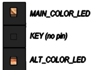
Figure 14 Alternate Power LED header
